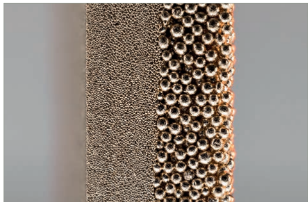
Bronze filters – SIPERM® B (Pore size 5 – 200 µm)
